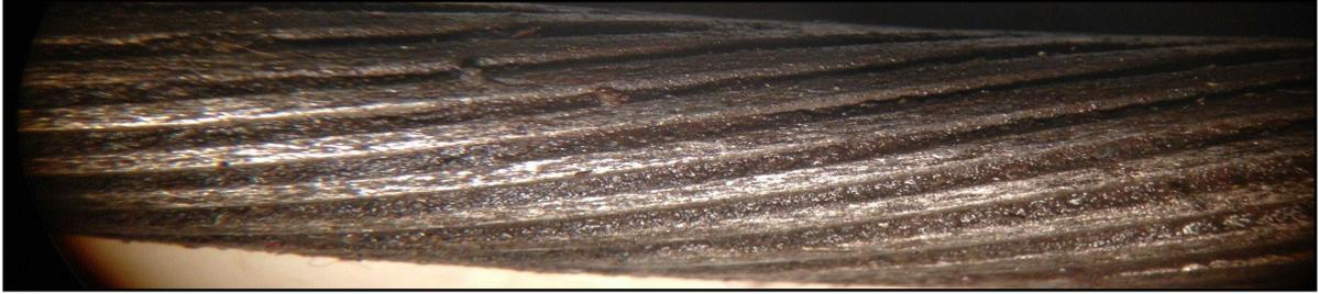
Another effect of damage due to loose armor can be seen in the picture below. This damage was most likely caused when it passed through the flow tube.
