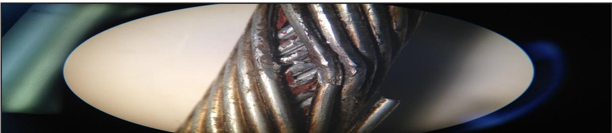
Examination of wireline for mechanical damage can be crucial in forensic analysis to determine its failure. As can be seen from the examples shown here, a lot of information can be obtained from the type of mechanical damage directly from handling the wireline, operations, operating environment, etc.
