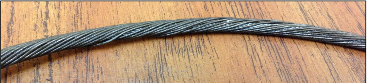
The picture shown below is from a crossed armor wire getting squeezed through a flow tube. The crossing of the armor wire probably occurred during re-heading and the crossed wire travelled all the way up to the flow tube and got jammed and broke.
