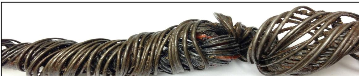
Abrasion of the outer armor by rubbing against a hard surface or incorrectly sized sheave can result in flattening effect on the outer armor. In the photo shown below it can be seen that the outer armor has flattened and is also affected by corrosion.
