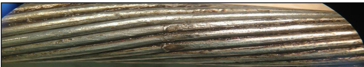
Loose cable, can lead to birdcages in the armor. This can happen if the cable is not serviced at regular intervals as recommended by the manufacturer. In the photos shown below it can be seen that excessive rotation under load has caused loose armor wires.
