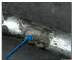
*Brass transfer is apparent due to galvanic corrosion.*
