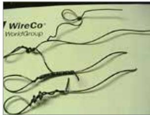
Wrap tests on four wire samples show no evidence of brittleness.
