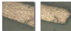
The armor wire ends from the cable side of the failures.
